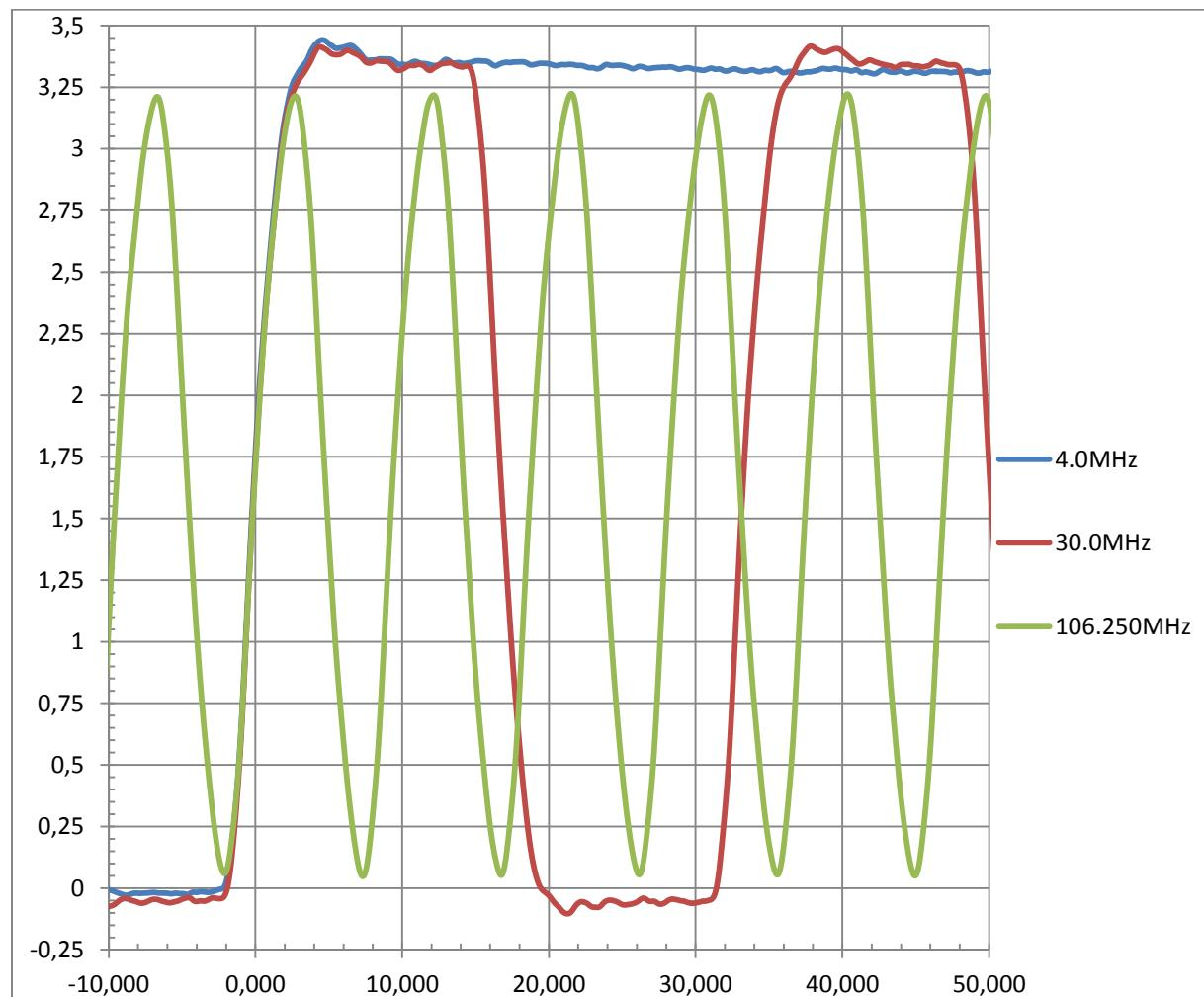
Example 2 - variation of rising / falling edge at constant load vs. Edge Control setting
