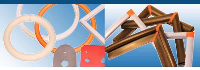
Jehbco Silicones is able to produce a large variety of O'Rings, from Silicone Cords or Silicone Strips. With Cross Sections from 1.0mm up to 40.0mm, and Diameters as large as needed. And Hardness's from 20 shore A up to 80 shore A. They are fabricated with a unique Vulcanizing technique which makes the joints as smooth as molded parts.
