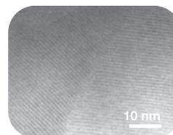
**Fig. 6** — STEM in SEM image of Faujasite showing 7.4 Å pore spacing.
