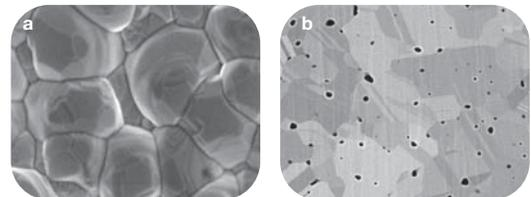
**Fig. 2** — Imaging top surface of a solar thin film: (a) as received; (b) after CP preparation, grain structure and porosity are clearly observed on the ion-polished surface.
