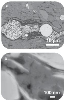
**Fig. 3** — (a) Backscatter SEM image of the CP prepared shale specimen taken using LABe detector. Dark contrast shows location of kerogen, white contrast shows pyrite crystals, gray contrast corresponds to areas of clay, carbonates and quartz. (b) nano-pores in kerogen-rich area.
