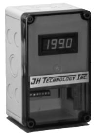
FDT5140/FDT5150 Multiply/Divide Transmitters respond to the product or ratio of two DC inputs and provide a proportional, isolated DC output. A rugged NEMA4X splashproof, corrosion-resistant housing protects the transmitter in outdoor and industrial environments. The circuit boards are urethane coated for protection against condensation and contaminants. FDT5000 Series transmitters include a 3-1/2 digit user-rangeable display to provide local process indication in engineering units.
