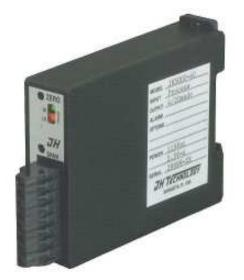
Model JH5200 provides a DC voltage or current proportional to millivolts produced by a thermocouple. Model JH5210 adds linearization to compensate for thermocouple nonlinearity, producing an output truly proportional to temperature. Both are fixed-range devices, precisely calibrated to your specified ranges at the factory.
