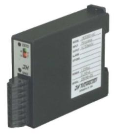
Model JH5600 and JH5610 AC Input Transmitters provide an isolated DC output proportional to an AC voltage or current input. Applications range from power monitoring to millivolt-level AC signals from sensors. Input/output isolation is standard to guard against shock hazards in power measurements and against ground loop errors. Inputs ranges may be zero based or may be expanded (for example, 50-150Vac).
