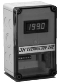
The Model FDT5800 Potentiometer Input Transmitter provides an isolated DC output proportional to the position of a potentiometer or slidewire wiper. The input range may be 0-100% or any 10% or wider portion of the wiper's travel. Calibration is unaffected by the potentiometer's end-to-end resistance.
