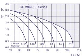
$\rm I_A$  = actual ripple current at 120Hz,  $\rm I_R$  = rated ripple current at 120Hz, 105°C Multiplier of Useful Life as a function of ambient temperature and ripple current load
