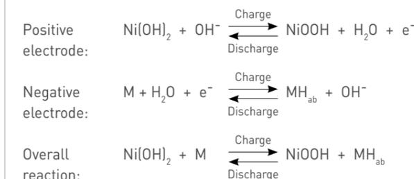
(M: hydrogen-absorbing alloy; H<sub>ab</sub>: absorbed hydrogen)
