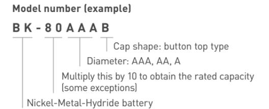
**STANDARD TYPE** Ni-MH battery technology is nowadays the Ni-Cd (Nickel-Cadmium) successor technology for rechargeable and portable devices. These batteries are ideal for less complex and cost sensitive applications. For example medical equipment and distance meter.
