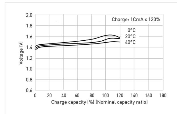
**Charge temperature characteristics at various charge rates**
