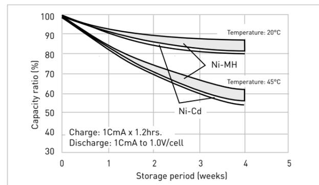
Self-discharge is affected by the temperature at which the batteries are left standing and the length of time during which they are left standing. It increases in proportion as the temperature or the shelf-standing time increases. Panasonic's Ni-MH batteries have excellent self-discharge characteristics.
