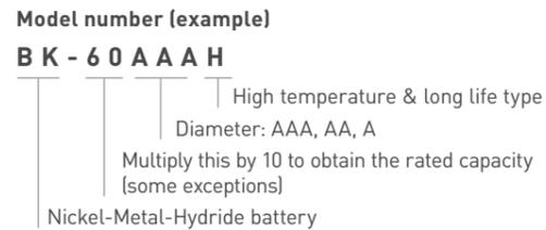
**HIGH RATE DISCHARGE & HIGH TEMPERATURE TYPE** These state-of-the-art back-up batteries deliver excellent current discharge characteristics at high temperature (60°C). They are able to power applications such as back-up for UPS, POS systems and solar window shutter.
