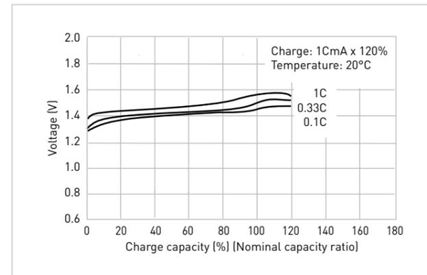
**Charge temperature characteristics at 1C charge**
