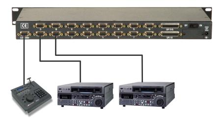
Connect your deck controller into the Controller port on the rear panel. Alternately, your deck controller can be plugged into the Controller port on the front panel if it is more convenient. In this case, make sure the front panel Enable button is illuminated.
