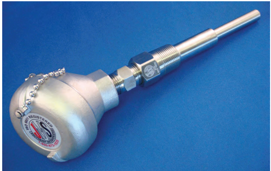
Step-shank thermowell assemblies provide a faster response to temperature change and are now within the scope of ASME 19.3TW.
