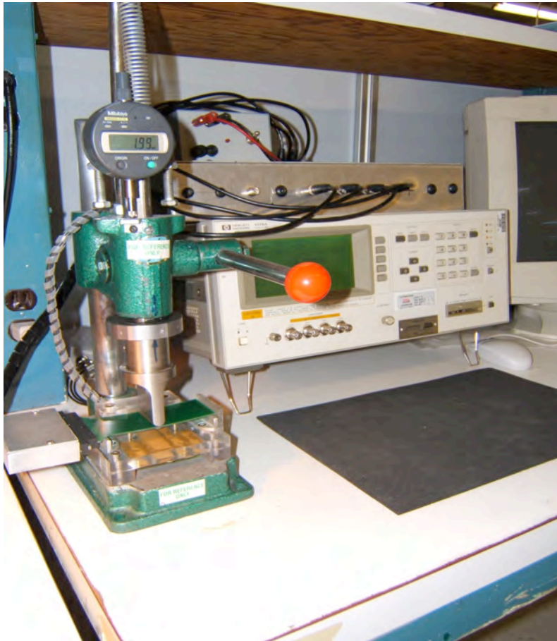
Figure 16 Flex Test Fixture W/CPU for Data Storage
