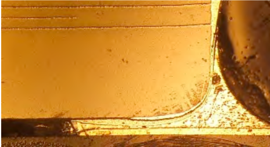
Figure 12 Partial Separation of Polymer 4mm
