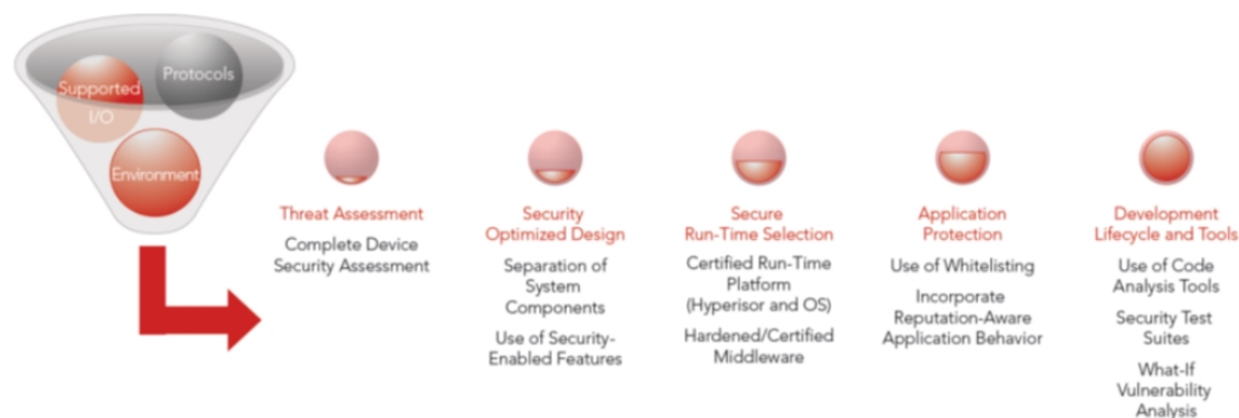
Figure 3: Steps to enhance automotive embedded security
