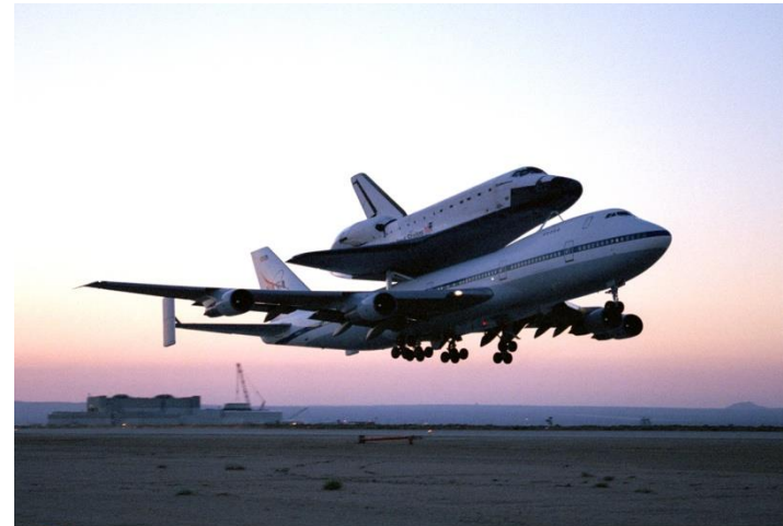
NASA Dryden Flight Research Center Photo Collection http://www.dfrc.nasa.gov/gallery/photo/index.html NASA Photo: EC02-0131-9 Date: June 28, 2002 Photo by: Carla Thomas The Space Shuttle Endeavour, mounted securely atop one of NASA's modified Boeing 747 Shuttle Carrier Aircraft, left NASA's Dryden Flight Research Center at Edwards Air Force Base in Southern California at sunrise on Friday, June 28.
