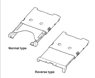
This is a tray type connector for the Micro SIM (Mini-UICC) card which downsized the conventional SIM card.
