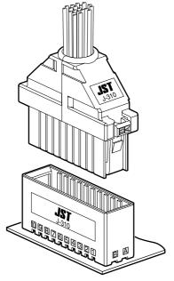
When applying a current to the connector, the protector prevents foreign substances being inserted into mating part from the wiring side. However it has no function of holding the wire securely.
