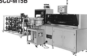
Auto. ID machines for 2.5 mm & 2.0 mm pitch jumper wires
