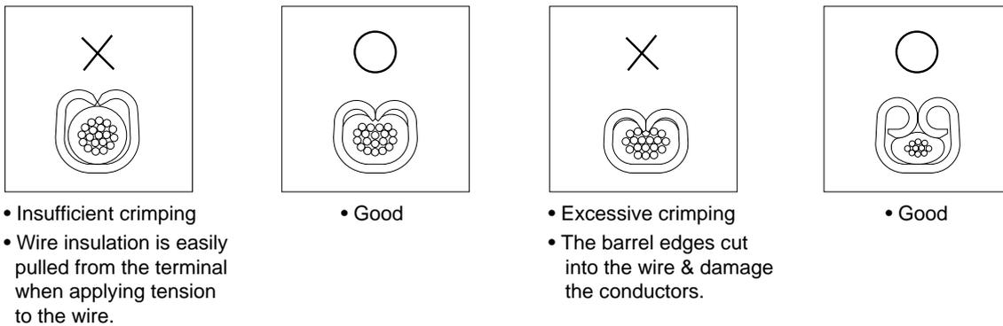
Check: Cut off the insulation support and remove the wire insulation, then check the wire conductors for damage.
