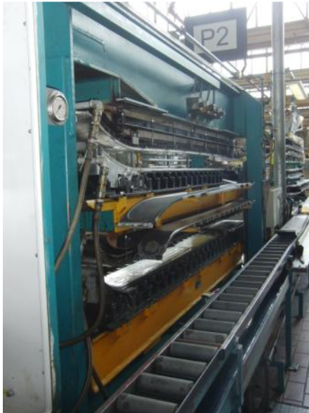
Fig. 2: Modern skis are "baked" in presses such as these
