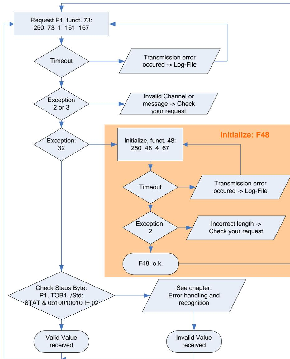
A simple example for reading out a pressure value. Because only one transmitter is connected, the „transparent“ address 250 is used. To read out pressure functions 73 and 48 are necessary. When the slave replies with error no. 32 (device just recently started up, power on), then this has to be confirmed with function 48. This is helpful to detect current supply interruptions (on the power supply circuit).
