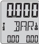
With the command EXE the new zero is being determined and stays as a reference until a new TARA is being executed or until the instrument is turned off.
