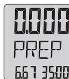
The test time is now programmed (35:00). The start of the leak-test is described on the next page.
