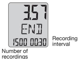
The display END indicates the end of the recording. Activate PREP to return to the PREP-Mode from the END display.
