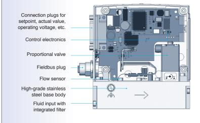
The mechanical connection between the pressure sensors and the main channel of the flow controller is implemented in each case with a capillary tube (vented by means of a de fined purging process), which is also de-signed as a lowpass filter for pressure peaks. All the parts that come into contact with the measuring medium (except for the sealing rings) are made of high-grade stainless steel.
