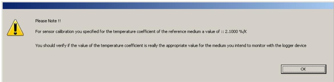
For correct calibration, the temperature coefficient of the test reference solution was required, but this value does not necessarily match with the physical properties of the water or medium you want to monitor with the logger device. Please verify the correct and appropriate temperature coefficient is stored in the device while running measurements on site.
