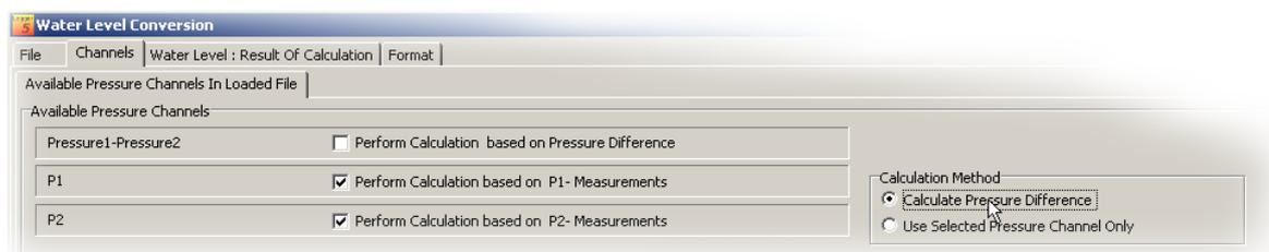
The other two check boxes "Perform Calculation on P1-Measurements" and "Perform Calculation on P2-Measurements" become then available.
