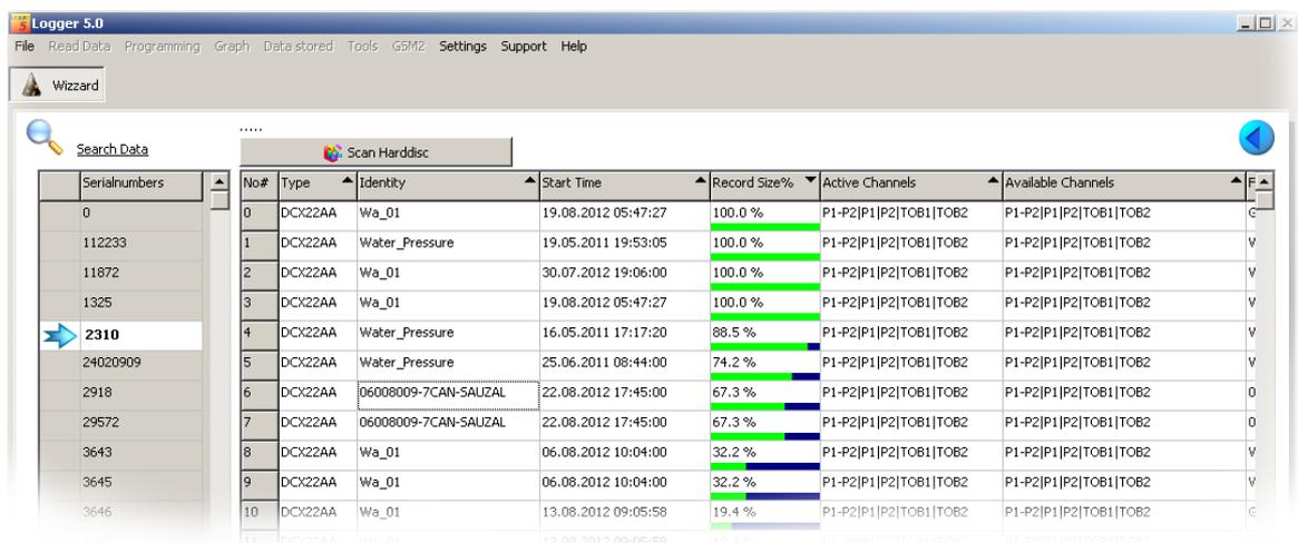
The grid on the left side displays the serial numbers of the logger devices. You may select a serial number to receive a table of all data files corresponding to the selected serial number.
