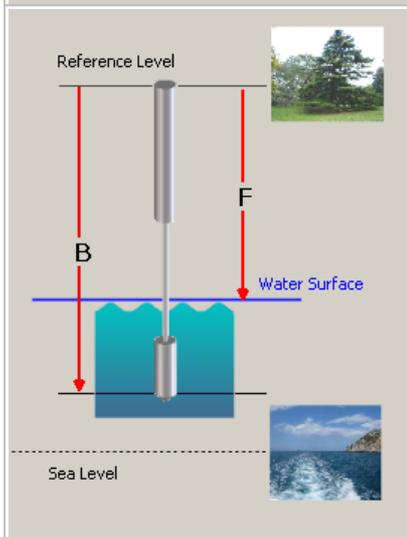
The water level is represented by the depth to water surface measured down from a reference level.
