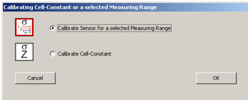
Two different options are offered for the desired calibration method.
