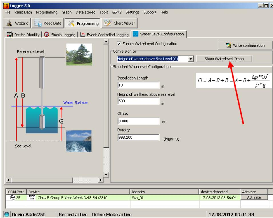
Press the button "Show Waterlevel Graph" to activate the window as shown in the figure below.
