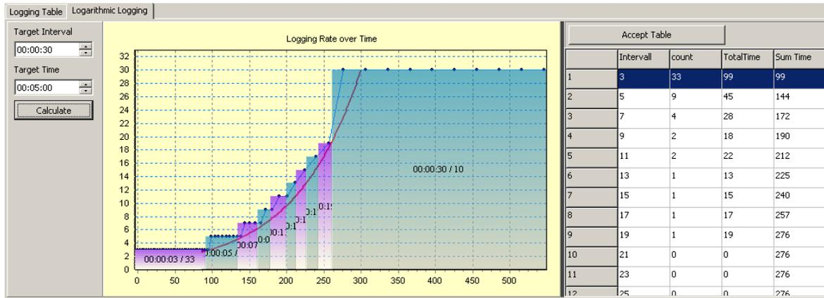
It's possible to specify a "Target Time" and a "Target Interval". These parameters set the logger device to collect data at the specified measuring time and at the specified fixed interval.
