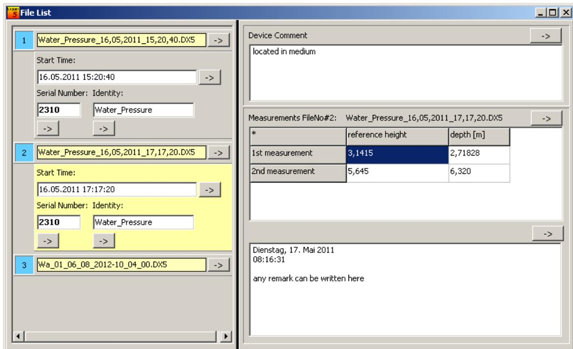
Using the arrow buttons
