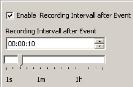
Recording is done at a fixed interval independent of Fixed Save-Interval. If Recording interval after event has been selected in addition to Event Detect Interval, the smaller of the two intervals applies.
