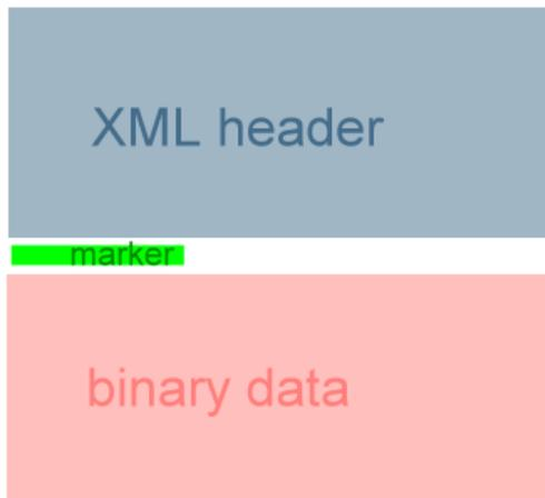
The XML header describing the logger device and its channels is separated by a marker from the binary data.
