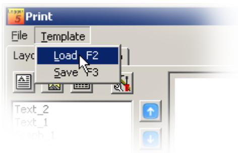
Use the main menu command "Template" -> "Load" to restore a previously designed page layout. Use "Template" -> "Save" to store the current page layout as template for later print jobs.
