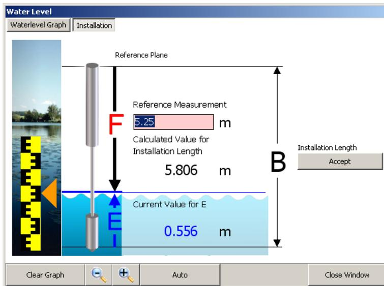
The red colored edit field allows to enter the manually measured depth to water **F**. Then press the button "Accept" to copy the calculated value for length **B**. You will find the value then in the field "Installation Length"
