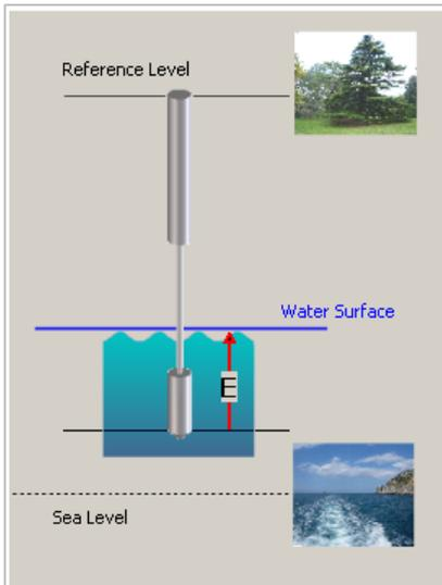
The water level is represented by the height of water column above the sensor.
