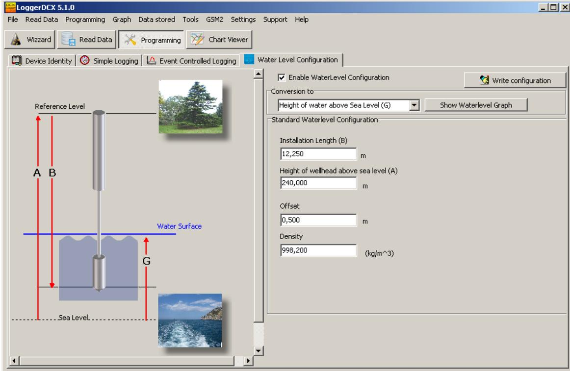
The screenshot shows the 'Water Level Configuration' dialog in the LoggerDCX 5.1.0 software. The dialog is titled 'Water Level Configuration' and has a 'Write configuration' button. It contains a diagram of a pressure sensor in a well with labels for 'Reference Level', 'Water Surface', and 'Sea Level'. The diagram shows two vertical lines, A and B, representing different levels. The sensor is labeled 'G'. The configuration panel on the right has the following fields:
