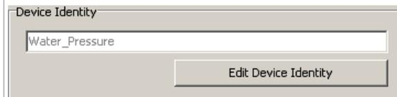
Press the "Edit Device Identity" button to change the field Device Identity.
