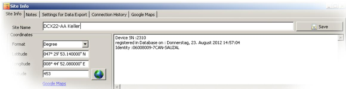
The comment field is automatically filled in "Device Serial Number", "Date and Time" and "Identity" stored in the device memory when the data file was registered in the database.
