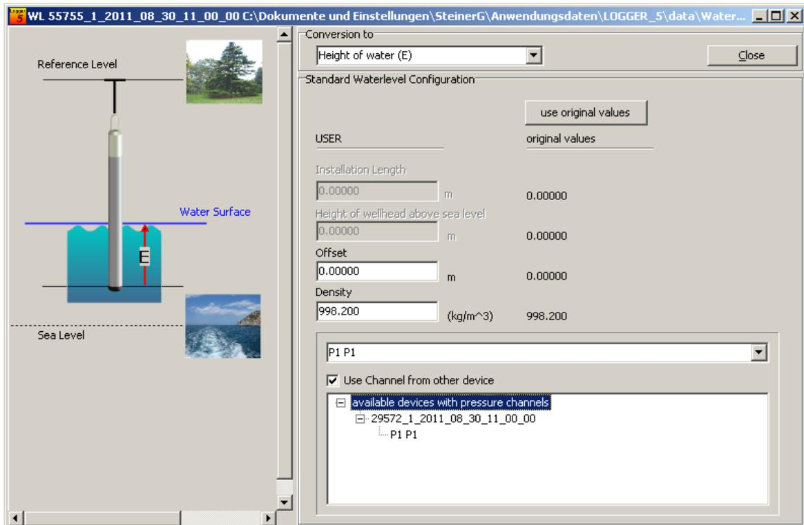
On the bottom right corner a tree view listing all available or currently loaded files allows to select any desired pressure channel. The checkbox "Use Channel from other device" is activated. You need to tell the Viewer from which device or file the barometric pressure should be derived from for water level calculation.
