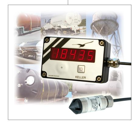
The Castello enclosure integrates an air pressure sensor, ranged between 0,8 bar and 1,3 bar absolute. The sensors to measure the hydrostatic pressure at the bottom of the tank are calibrated from 0,8 to 1,8 bar abs for tanks up to 5 m in height, and 0,8 to 2,3 bar abs for tanks up to 10 m in height. The pressure difference, calculated by the  $\mu$ P, is the relative hydrostatic pressure.
