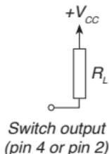
PNP switch output with external load ( $R_L$ )
