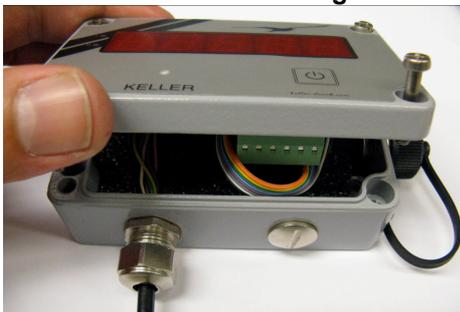
Close the housing and install the four screws.
