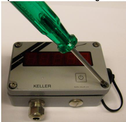
Remove the four screws on the front panel.
