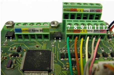
Connect the cable ends to the terminal strip (transmitter 1).
