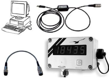
Connect the Castello to the PC using converter cable K104-B (USB) or K107 (RS232). Cable option 5 must be used between the Castello and the converter cable.
