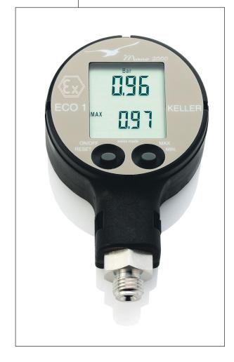
ted temperature range from 0 to 50 °C, the economically priced standard manometer offers typical overall accuracy of 0,5 %FS (Full Scale). The standard design features IP65 protection, and the optional protective cover means that it can also be operated reliably outdoors in any weather conditions. This instrument is also available in an Exia ATEX approved version compliant with 94/9/EC.
