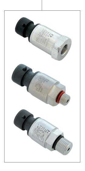
Output signals with different voltage and current formats are available for any application area, be it in cars or industrial environments. The supply voltage can be either 5 V (fixed) or 8 to 28 V (variable). The electrical connection is compatible with the Packard connector that is a standard used in the automotive industry.
