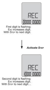
After setting the number of recordings, set the recording interval in min:sec in the same way. The adjustment of the storage parameters can be terminated by activating PREP.
