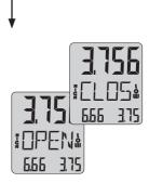
The pressure switch opens. The status and the switch pressure are displayed.
