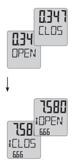
The pressure switch closes. The status and the switch pressure are displayed.
