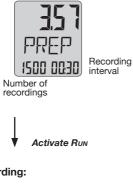
The display END indicates the end of the recording. Activate PREP to return to the PREP-Mode from the END display.
