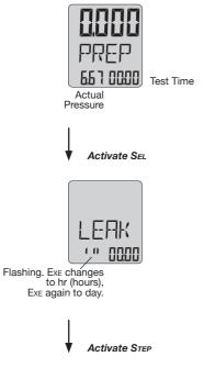
When the test time is set, activate PREP. The display is now back in PREP-Mode.
