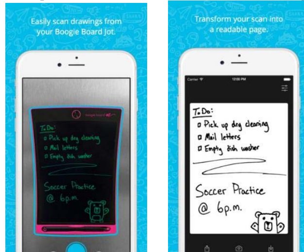
Fig. 14: Boogie Board Jot 8.5 app allows note saving. Jot app takes a photo of device and inverts image to black writing on a white background.
