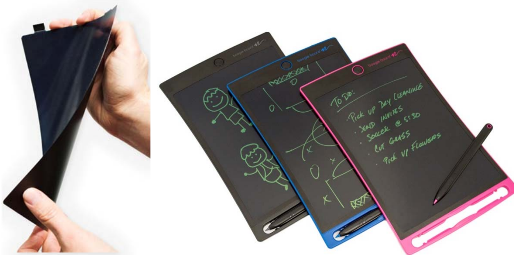
Fig. 1. (On Left) A photograph of a flexible eWriter display. (On Right) A photograph of a Boogie Board Jot 8.5 that allows electronic erasing of handwritten notes.
