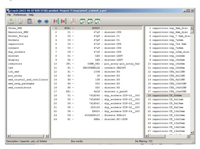
The left pane contains the list of available footprint library file names associated with the project. The center pane contains the list of components loaded from the net list file. The right pane contains the list of available footprints loaded from the project footprint libraries. The component pane will be empty if no netlist file has been loaded and the footprint pane can be also empty if no footprint libraries are found.
