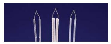
The Process Probe 1530 is designed for use in a variety of equipment configurations, spanning a wide range of temperatures (0 °C to 1,100 °C). All thermocouple leads are safely insulated for a specific temperature range, using either low-particulate quartz microtubing or highly flexible braided silica sleeving for high temperatures, or polyimide coated insulation for lower temperatures.
