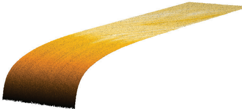
Roll Off: Sapphire edge profile; 5x1 FoV stitched with a 5x objective
