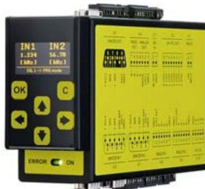
Safety-M Compact: Safe speed monitoring allows for a wide range of drive functions – thanks to the free choice of incremental encoders.
