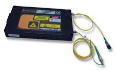
with a diffraction-limited beam (output fibre with  $M^2 < 1.5$  for energy above  $15\mu$ J), and is available as a benchtop unit with user friendly interface or modules. The modules are compact, robust devices that are maintenance free with high reliability, so are ideal for integration into a complete optical system.
