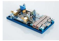
available is tight. High power modules incorporate built-in base plate heat sinks as standard and all drivers are compatible with most typical package types associated with common pulsed laser diodes.
