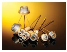
A range of options is available to suit requirements for varying emitter stripe widths and package design.
