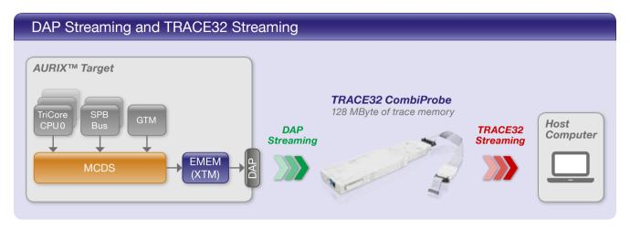
Lauterbach has been supplying its new CombiProbe TriCore DAP for the AURIX™ family from Infineon since October 2016. This means TRACE32 now offers comprehensive run-time analyses for all AURIX users whose target hardware does not provide an AGBT interface.
