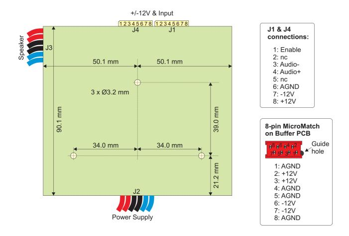
The drawing is from top (looking down at the module, mounting plate under the module) and can be used as drilling template.
