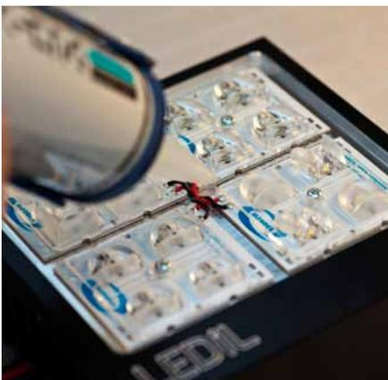
Apply potting compound only outside the optical area. Lens is designed with barrier walls to keep the compound out of the lenses.
