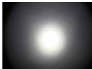
Reflectors produce much softer cutoff even if the viewing angle is same.
