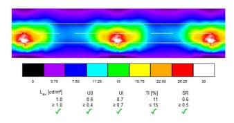
1) ME3a Street refers to a street lighting setup designed to pass ME3a requirements on EN 13201 standard.
