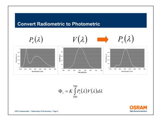
This slide shows graphically the radiometric spectral power distribution, P sub e, multiplied by the photopic curve V-lambda. By taking the area under the resulting P sub v curve and multiplying by the constant K, the luminous flux in lumens is calculated.
