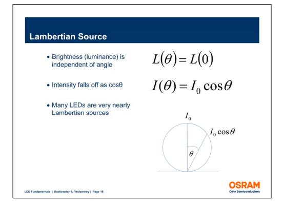
A Lambertian source is defined as one in which the brightness (or luminance) is independent of angle – in other words, the off-axis luminance is the same as on-axis. Such a source has an intensity versus angle profile that falls off as the cosine of the angle. Historically, many LED sources have had nearly Lambertian beam distributions, simplifying certain calculations.
