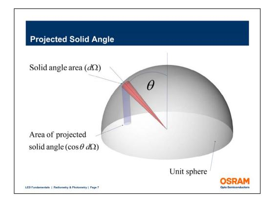
Projected solid angle takes into account the projected area when the viewpoint is other than the center of the sphere. The element of solid angle is shown in red. The area of projected solid angle is shown in blue.
