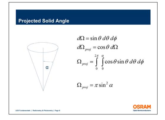
As an example, the projected solid angle for a cone of half angle alpha is calculated.
