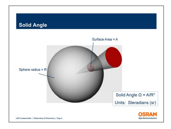
Solid angle is the 3 dimensional analog of an ordinary angle. In the figure, the edge of a circular disk, the bright red circle, is projected to the center of a sphere. The projection intersects the sphere and forms a surface area A.
