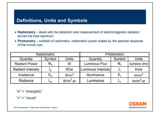
The table summarizes the most common radiometric and photometric quantities.
