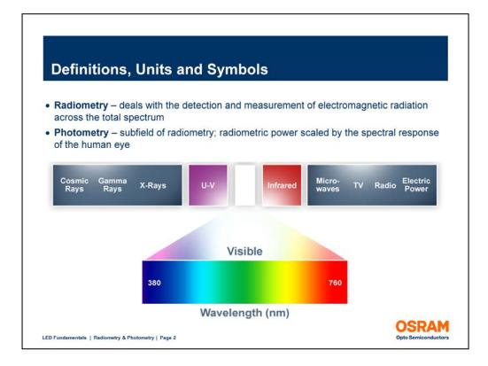
Radiometry is the field which deals with the detection and measurement of radiation across the full electromagnetic spectrum, including ultraviolet, visible, and infrared radiation. Photometry is concerned only with the visible portion of the spectrum, from about 380 to 780 nanometers.
