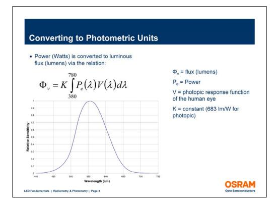
Radiometric power is converted to luminous flux via the integral equation. Vlambda is the spectral response of the human eye in daylight, otherwise known as the photopic curve. The unit of luminous flux is the lumen.
