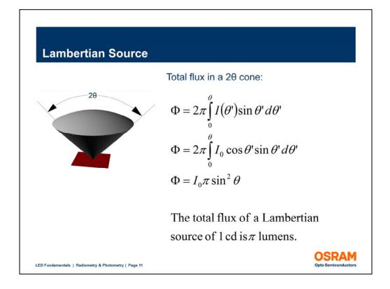
Take the example of calculating the luminous flux within a certain cone angle. Substituting the intensity distribution of a Lambertian source into the equation makes the integration simple. For a so-called Lambertian LED, the total lumens is about three times the on-axis intensity.
