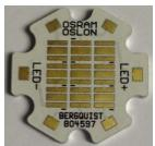
Standard metal core star board for 3x3 cluster. Nine OSLON LEDs are tightly clustered to increase light output nine times that of a single OSLON. This board is ideal for testing and prototyping of applications that require higher flux, but have tight spacing requirements.
