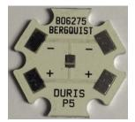
Standard metal core star board that can be used for testing and prototyping purposes on multiple HB LED applications with DURIS P 5 LEDs.
