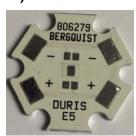
Standard metal core star board that can be used for testing and prototyping purposes on multiple HB LED applications with DURIS E 5 LEDs.
