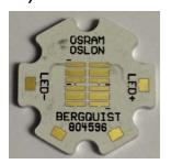
Standard metal core star board for 2×2 cluster. Four OSLON LEDs are tightly clustered to increase light output four times that of a single OSLON. This board is ideal for testing and prototyping of applications that require higher flux, but have tight spacing requirements.
