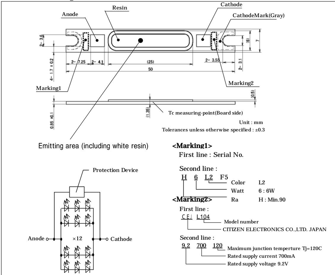
It has a protection device built in as a protection circuit against static electricity.
