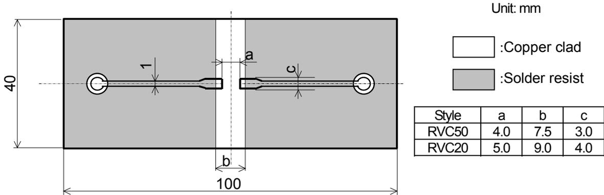
RVC50,63 TERMINAL STRENGTH TEST SUBSTRATE
