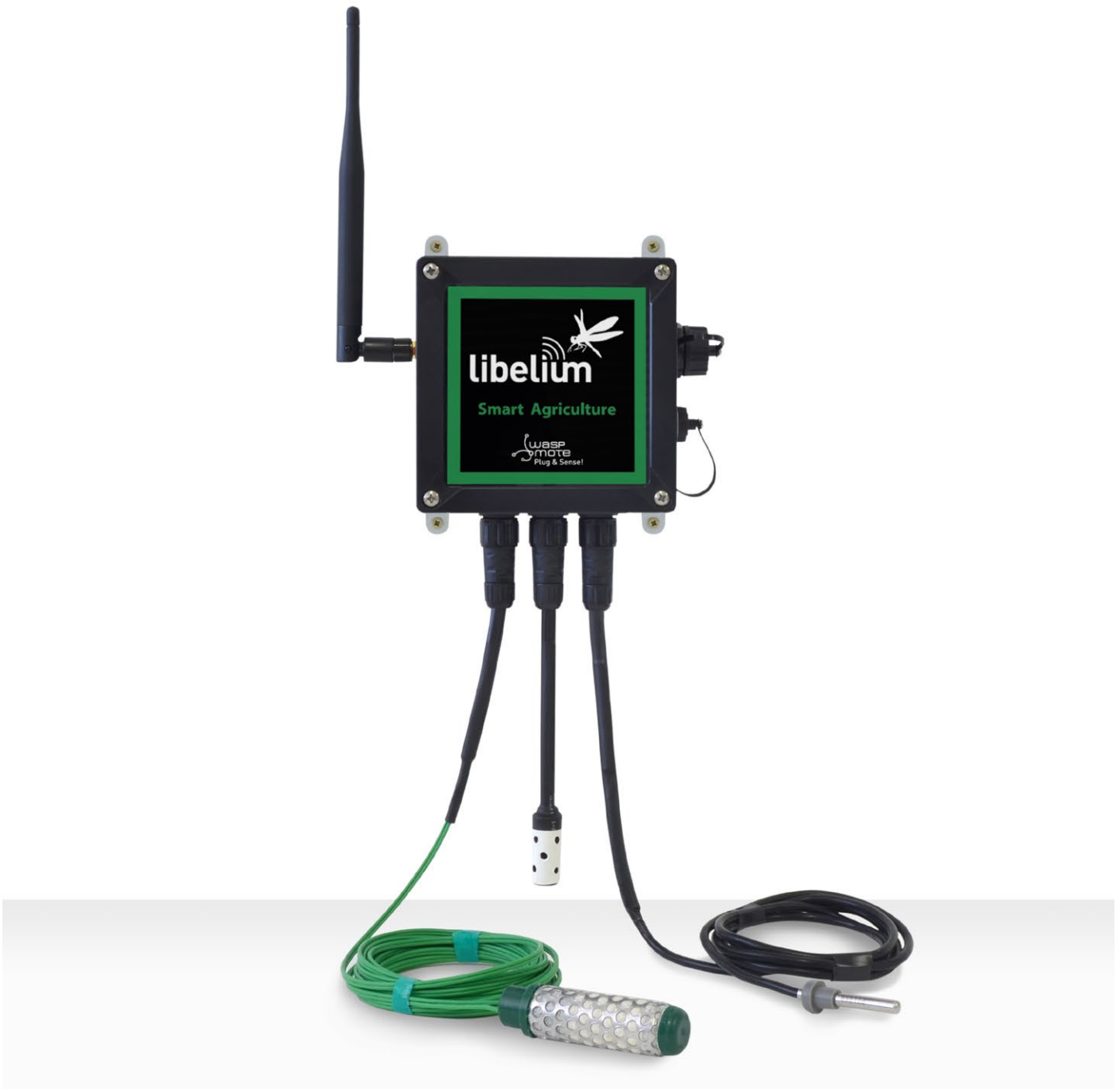
Figure : Smart Agriculture Waspote Plug & Sense! model
