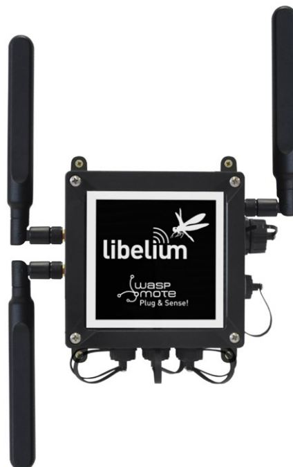
Figure : Plug & Sense! 4G, with 3 antennas
