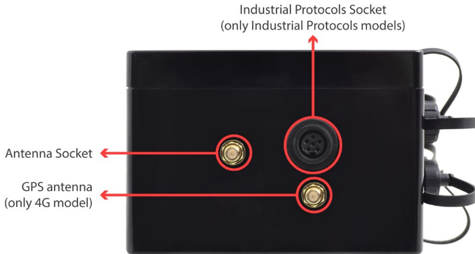
Figure : Antenna side of the enclosure
