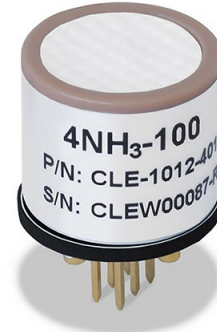
Figure : Image of the Ammonia Sensor mounted on its AFE module
