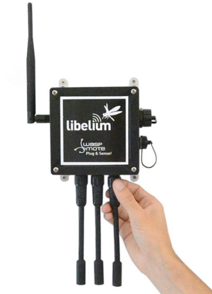
Figure : Connecting a sensor probe to Waspote Plug & Sense!
