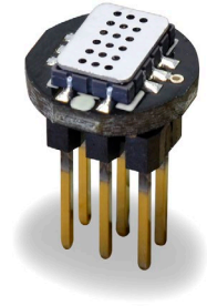
Figure : Image of the MiCS-2614 sensor
