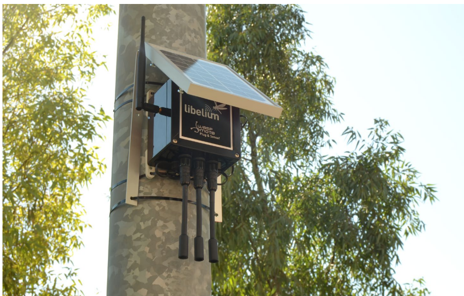
Figure : Waspote Plug & Sense! powered by an external solar panel
